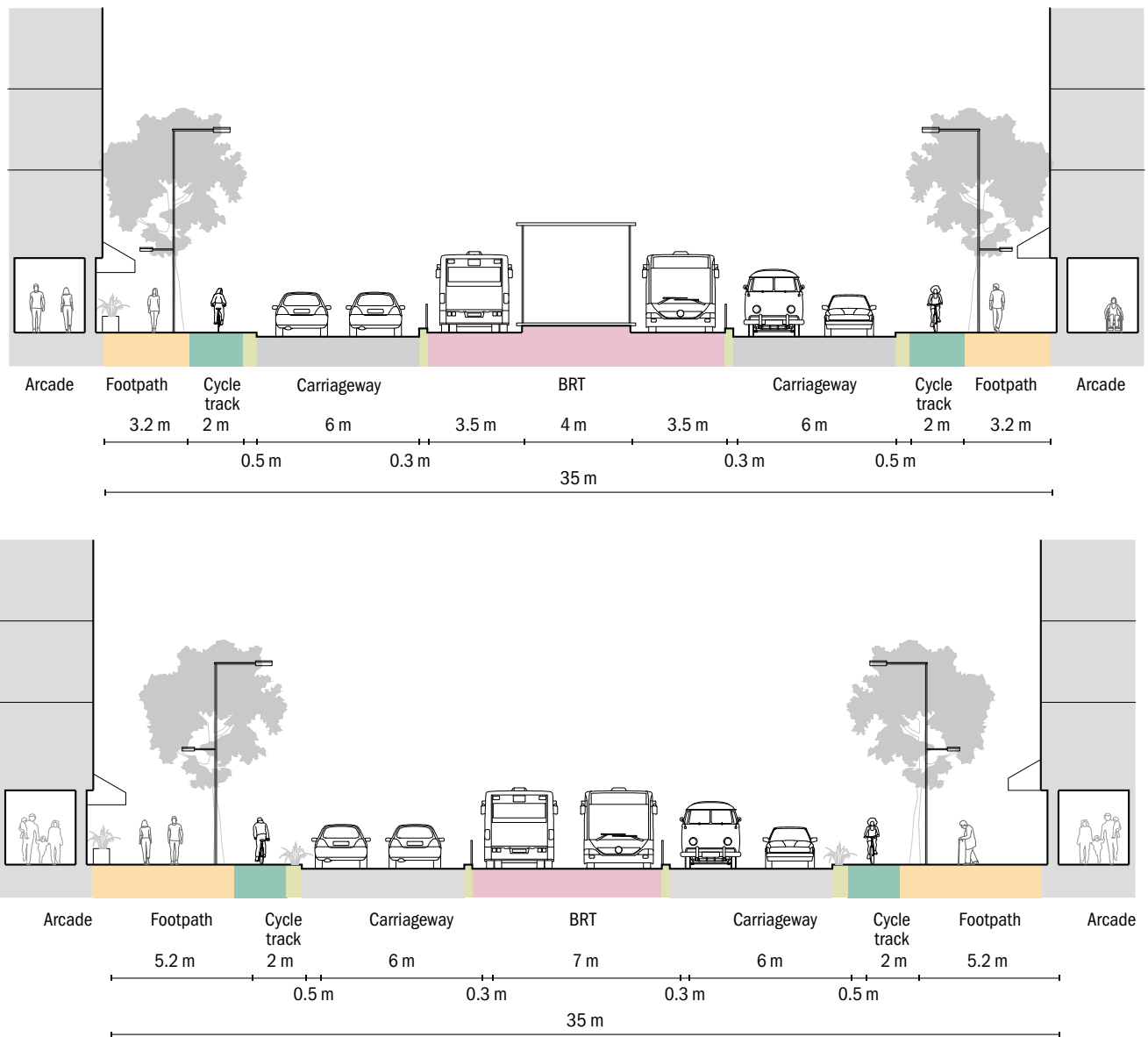
Figure 49. This typical BRT alignment with a single lane per direction can accommodate passenger volumes of up to 6,000 passengers per hour per direction (pphpd) with 12 m buses and 10,000 pphpd with articulated buses.
