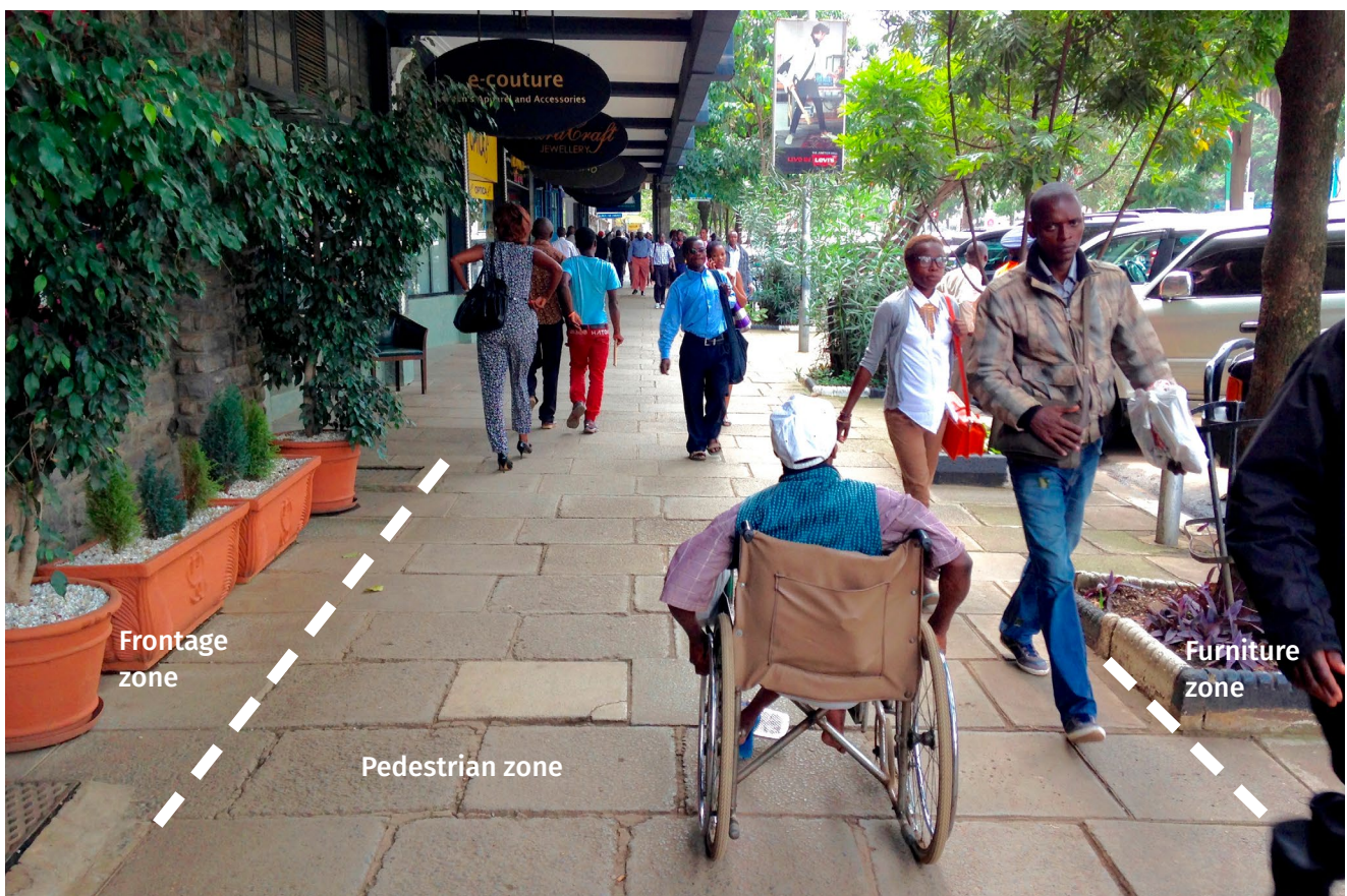
Figure 20. Footpaths designed per the zoning system provide uninterrupted walking space for pedestrians. The pedestrian zone should have at least 2 m of clear space.
