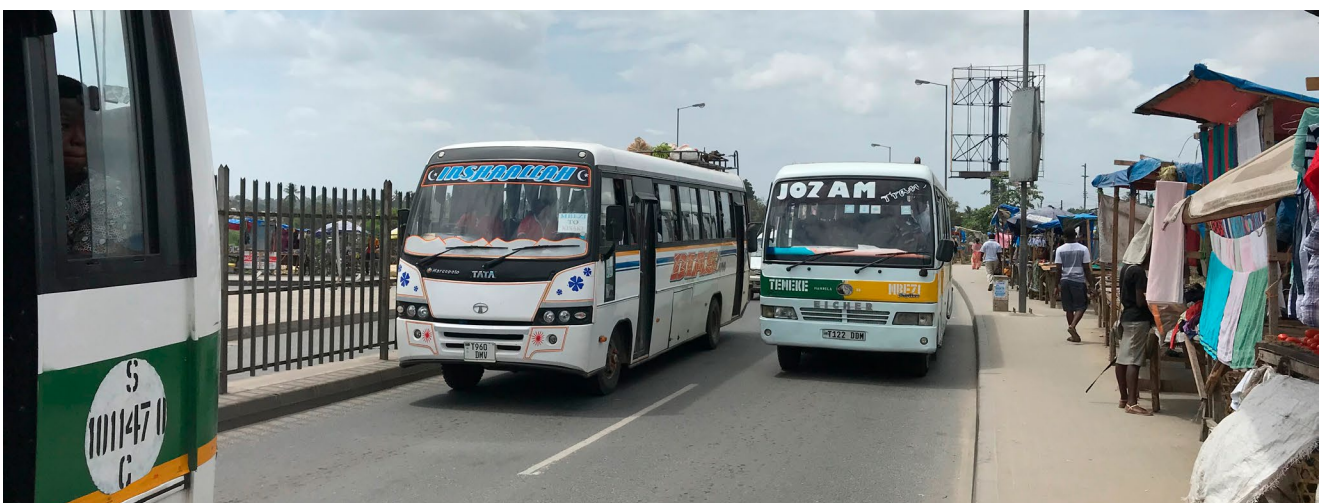
Figure 54. In urban areas, 3.25 m lanes can accommodate movement of large vehicles at moderate speeds.
