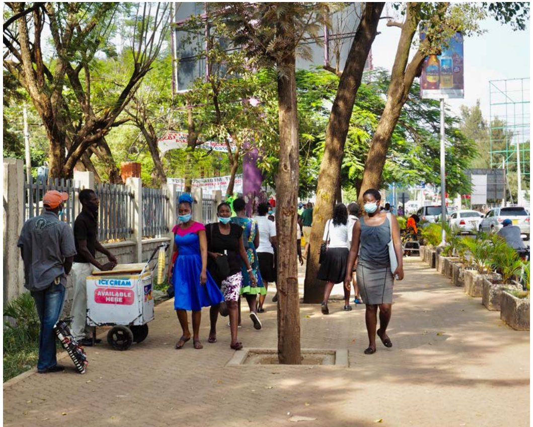
Figure 59. Footpaths should be designed such that there is sufficient space for vending outside of the pedestrian zone.
