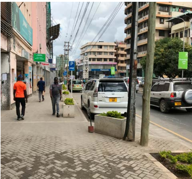
✓ Figure 69. Parallel parking for cars is preferred over angular or perpendicular parking because it saves space and is safer while exiting the parking bay. The standard width for a parallel parking lane is 2.2 m in commercial areas and 2.0 m for taxi stands. Larger parking slots can be provided for persons with disabilities.
