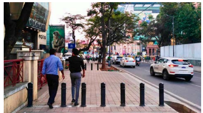
Figure 25. Bollards should be installed to prevent vehicles from parking on footpaths, with spacing of 900 mm between at least one set of bollards to allow wheelchairs to pass.
