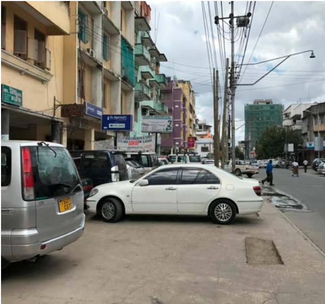
✗ Figure 70. Angular and perpendicular parking occupy a large portion of the right-of-way. Exiting the parking bay can be dangerous because drivers have limited visibility.
