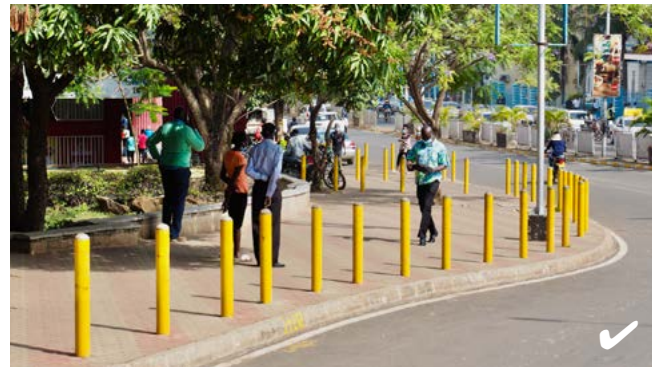
Figure 24. Footpaths placed below the carriageway often experience waterlogging. Footpaths should be raised +150 mm above the carriageway. A cross slope of 2% is required.
