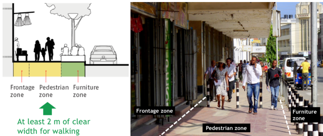
Figure 64: A well-designed footpath has three main zones: the frontage zone; pedestrian zone, with a minimum clear width of 2 m; and the furniture zone.
