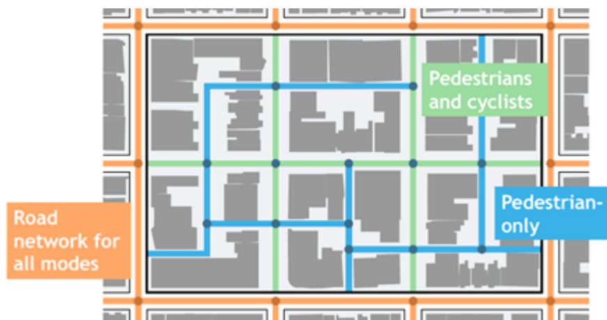
Figure 85: A fine-grained network of streets improves access for NMT users.
