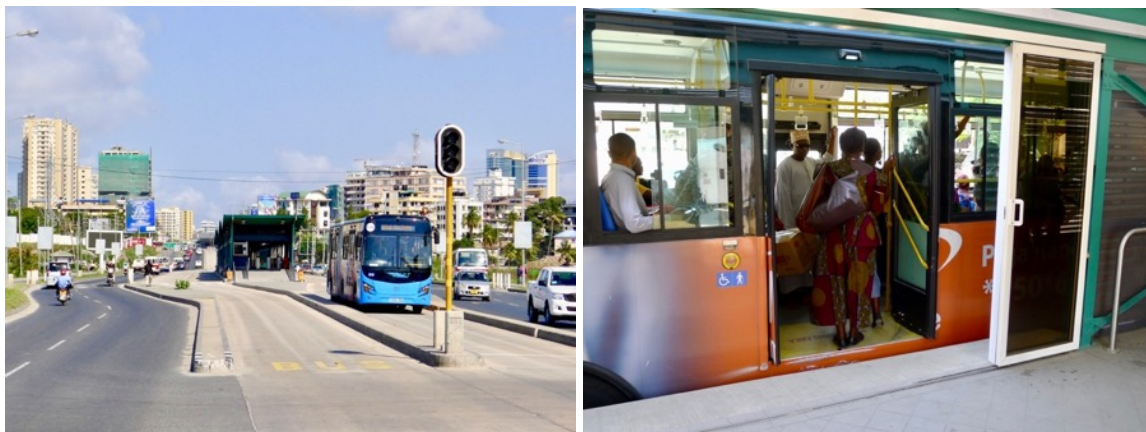
Figure 81. BRT systems, such as the Dar es Salaam BRT system pictured here, incorporate features such as dedicated median bus lanes and level boarding from central stations.
