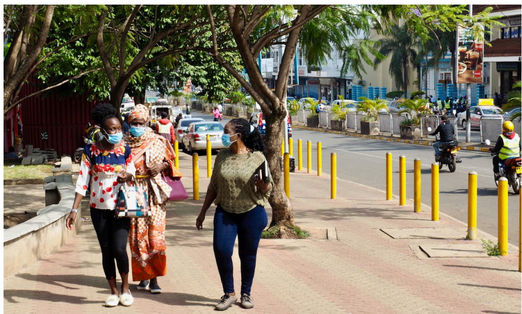
Figure 4. Bollards prevent vehicles from accessing footpaths.
