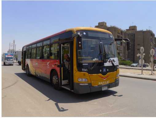
Figure 3. The Cairo Transport Authority (CTA) operates buses across routes in Cairo, Giza, and the new communities. The entire fleet consists of high floor buses with stepped entry.
