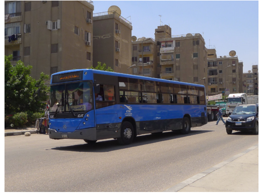
Figure 3. The Cairo Transport Authority (CTA) operates buses across routes in Cairo, Giza, and the new communities. The entire fleet consists of high floor buses with stepped entry.
