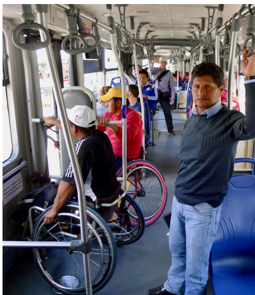
Figure 37. All public transport vehicles require ample space on board for wheelchairs. Vehicles providing service at the kerbside require ramps or lifts.
