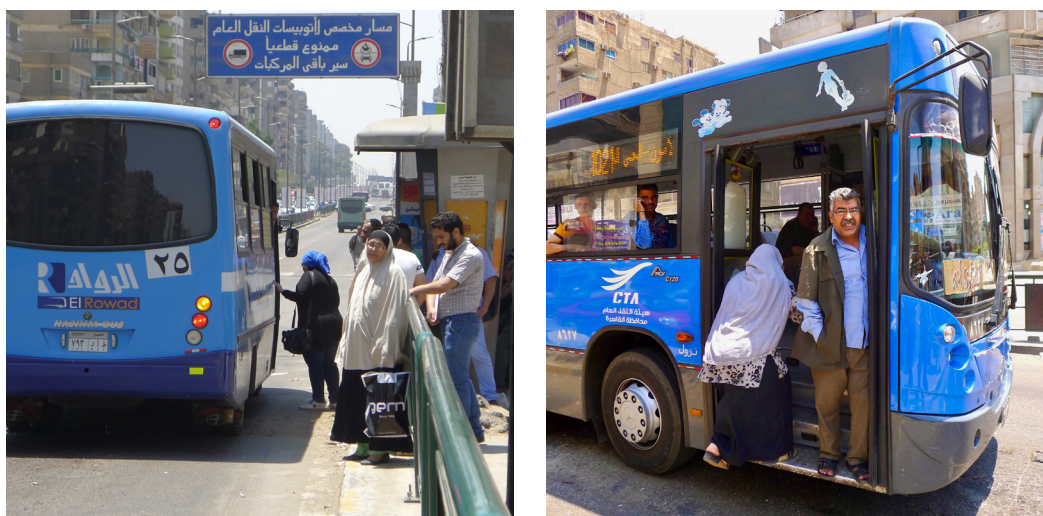
Figure 22. Steps inside buses and minibuses present a challenge during boarding and alighting, especially for elderly passengers, persons with disabilities, and caregivers with children.
