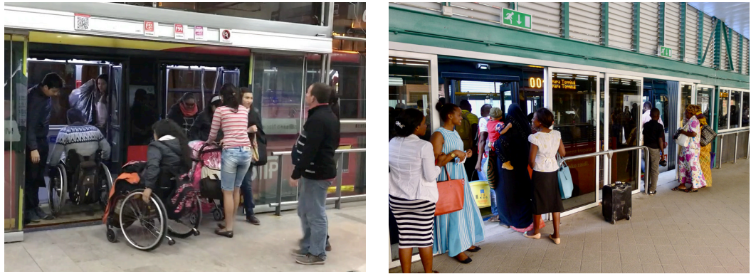
Figure 34. BRT stations should incorporate level boarding to ensure seamless access between stations and vehicles.
