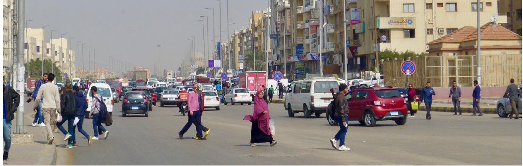
Figure 29. At several locations, pedestrians are forced to navigate wide crossings that lack signals or traffic calming.
