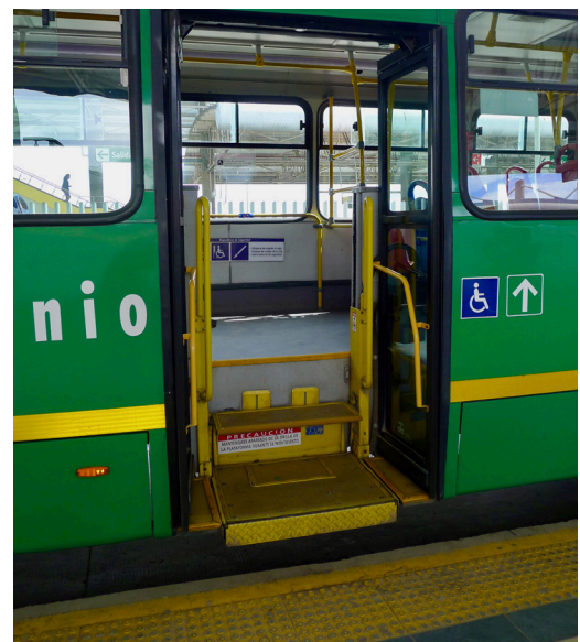
Figure 37. All public transport vehicles require ample space on board for wheelchairs. Vehicles providing service at the kerbside require ramps or lifts.
