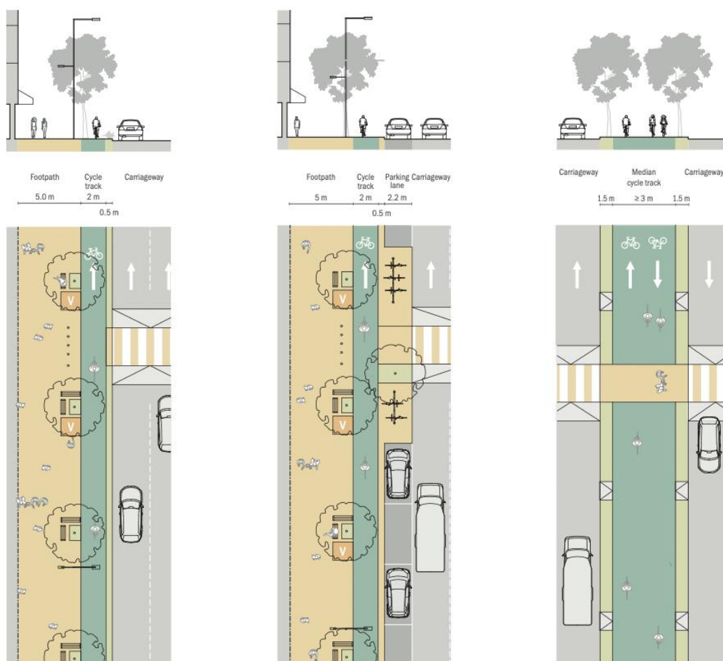
Figure 47. For one-way movement, cycle tracks should have a width of 2 m plus a 0.5 m buffer next to the carriageway. The width should be increased to 3.0 m for two-way movement.
