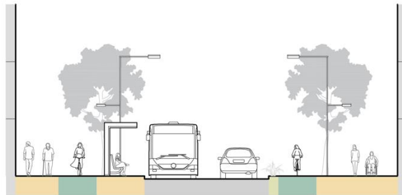
Cycle track Carriageway Cycle track Footpath
