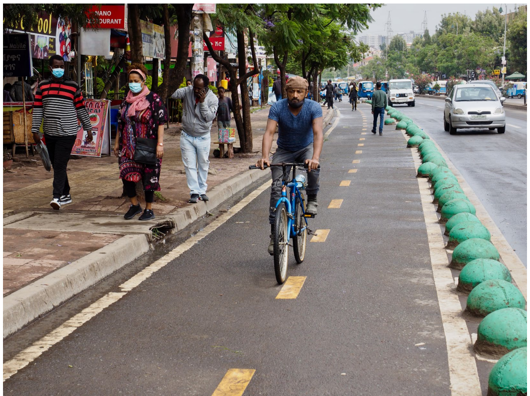
Figure 36. Part of an oversized carriageway can be re-purposed as a cycle track. Physical separators protect cyclists from motor vehicle traffic.
