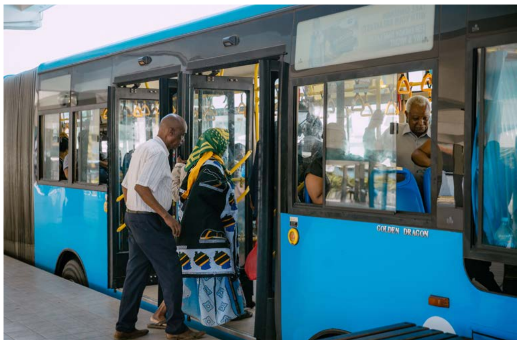
Figure 9. Level boarding allows for ease of movement and reduces the amount of time that the bus needs to remain stopped at stations.
