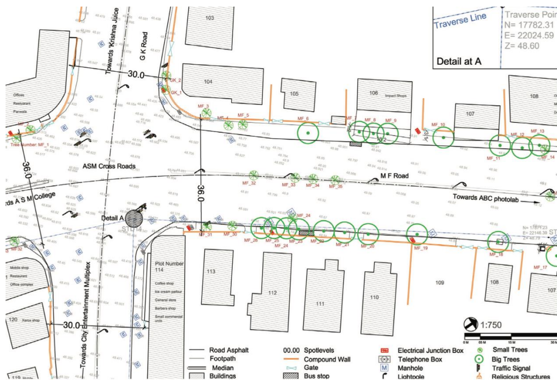
Figure 63. Sample topographic survey drawing.
